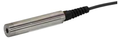
Calibration-free measuring sensor for dissolved oxygen according to the luminance method. Digital value transmission to the controller. No interference by  $H_2S$ , reducing or oxidizing substances. Evaluation via display unit. The dissolved oxygen sensor is available with a 10 m or a 2 m fixed cable.
